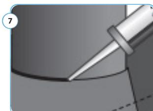
Seal the top of the collar with a weather-resistant silicone.
