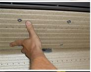
Remove the baffle plate by lifting it upwards and tilting on end.
