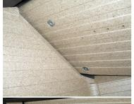
The flue ways are consist of a baffle plate and a smoke conductor above. This parts are screwed together. Both parts are made of vermaculite. Handle these parts carefully.
