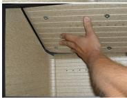
Lift the baffle plate a little and push towards one of the sides.
