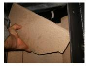
Then remove the smoke chicane by lifting up and tipping it backwards. Carefully lift out the smoke chicane.
